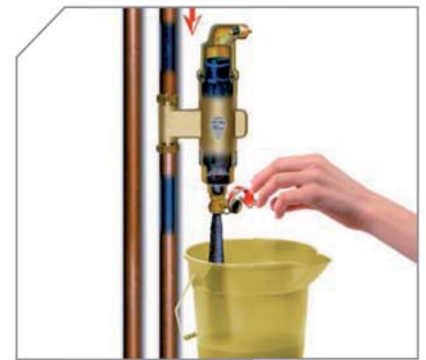
▷ 2: After one year**: open the drain valve for 3-5 seconds until the water is clear
